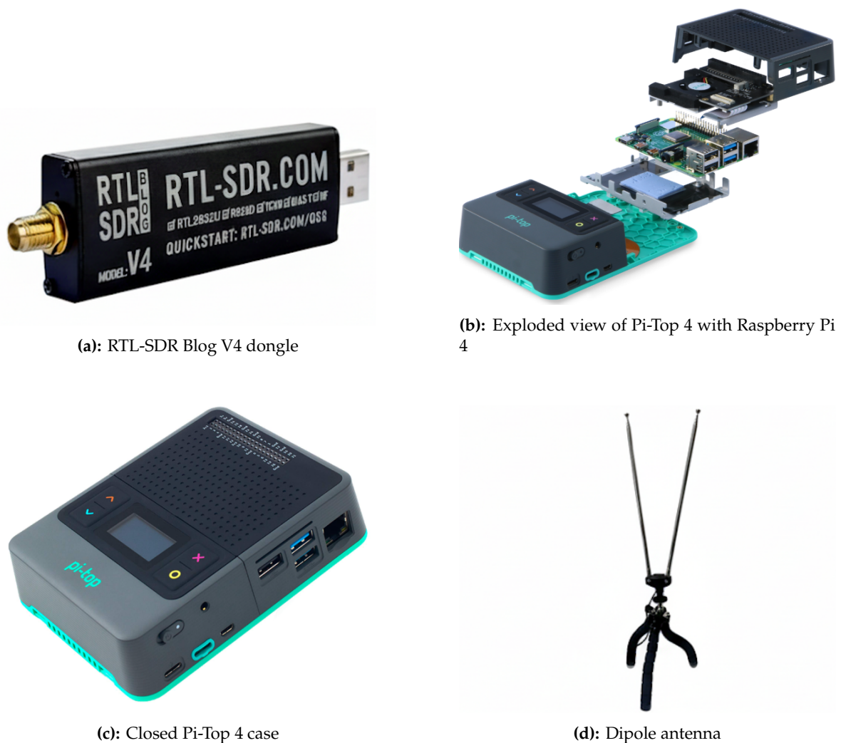
Figure 1: Hardware components used in the SDR receiver project: RTL-SDR Blog V4 dongle, Pi-Top 4 (exploded and closed), and dipole antenna.
